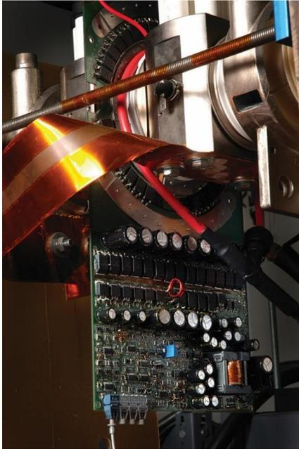
**3. A solid transformation.** For a decade now, North Carolina State University’s FREEDM Systems Center has explored how solid-state transformers (SST)—essentially a collection of high-powered semiconductor components, conventional high-frequency transformers, and control circuitry—can provide flexibility to the grid. *Courtesy: North Carolina State University*
